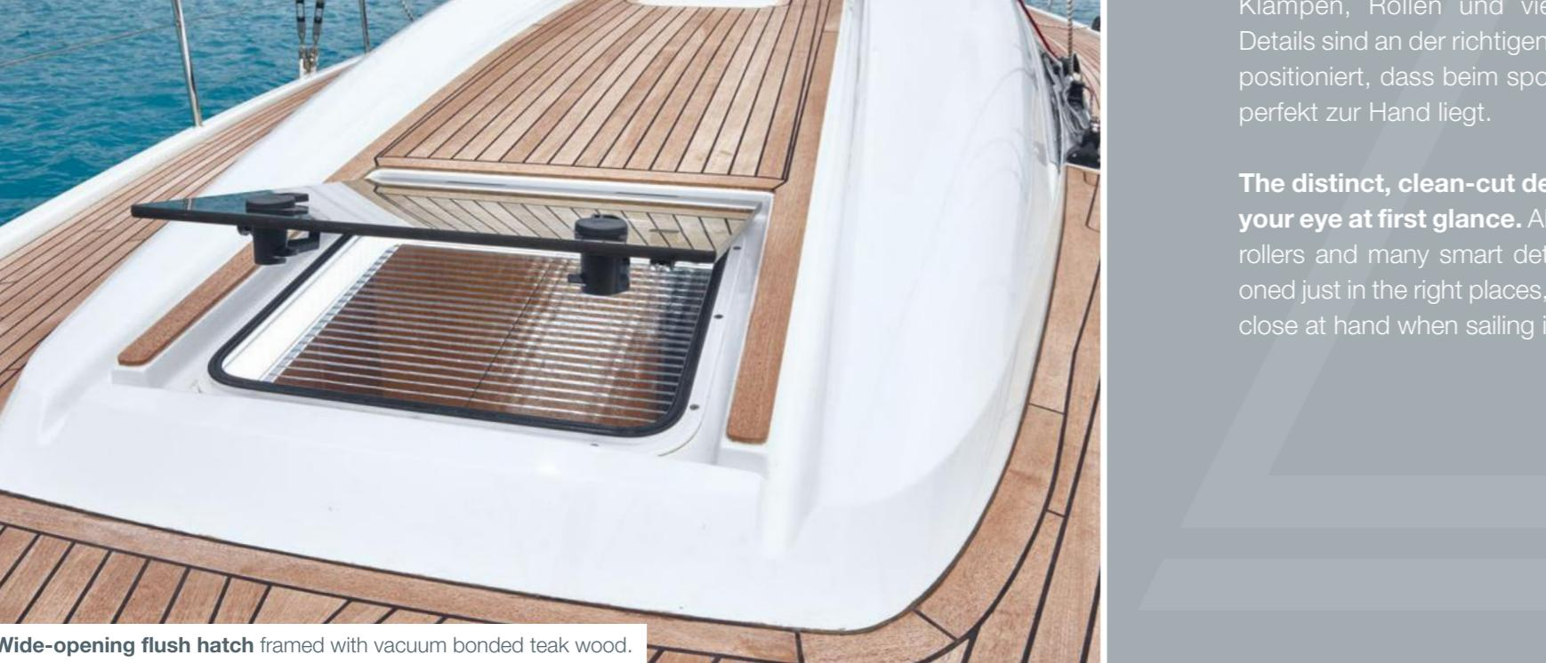
**Wide-opening flush hatch** framed with vacuum bonded teak wood.
