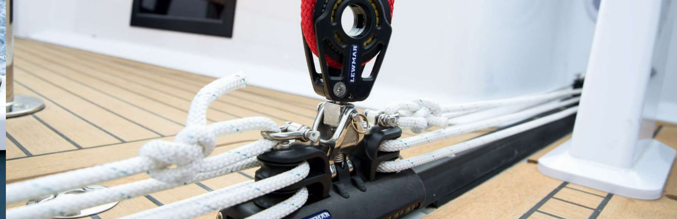
Being recessed into the floor, the mainsheet traveller allows an ideal trim of the mainsail.
